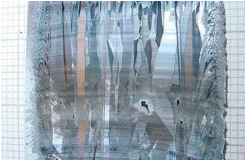
Fig.3. Top view of a SDS ribbon after the final ZMR step. The ribbon is 3 cm wide and the thickness is 300 \mu\text{m} .
