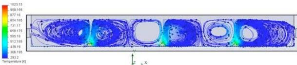
Fig. 6. Computational Fluid dynamics (CFD) analysis of the convection flows inside of the reactor. The reactor cavity dimensions are 20 mm x 60 mm x 300 mm. The ratio between the distance from the sample to the quartz window and the distance between heat regions (80 mm) is 1/4. The fluid injection is made from the orifice on the left wall. (Reactor side view)
