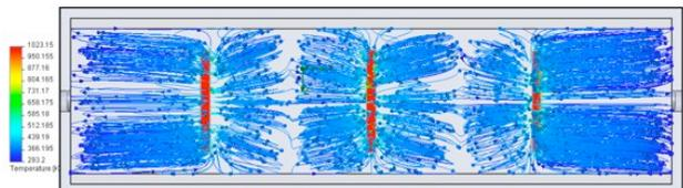
Fig. 8. Computational Fluid dynamics (CFD) analysis of the convection flows inside of the reactor. The reactor cavity dimensions are 40 mm x 70 mm x 300 mm. The long lateral walls are adiabatic. (Reactor top view)
