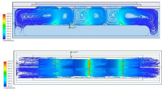
Fig. 3. Computational Fluid dynamics (CFD) analysis of the convection flows inside of the reactor. The convection flows result from the heating zones (red stripes) and the geometry of the reactor. Reactor side view (top) and top view (bottom). The ratio between the distance from the sample to the quartz window and the distance between hot regions is 1/2.
