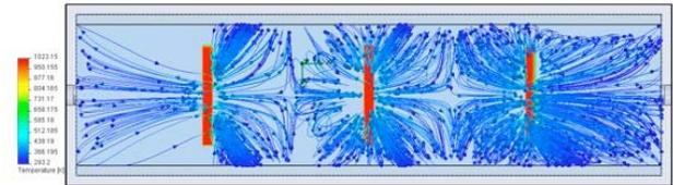
Fig. 7. Computational Fluid dynamics (CFD) analysis of the convection flows inside of the reactor. The reactor cavity dimensions are 40 mm x 70 mm x 300 mm. Whole the cavity is from aluminum cooled at 293.15K (Reactor top view)
