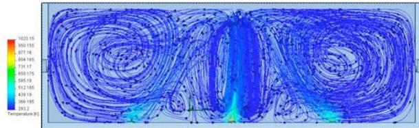
Fig. 5. Computational Fluid dynamics (CFD) analysis of the convection flows inside of the reactor. The reactor cavity dimensions are 90 mm x 60 mm x 300 mm. The ratio between the distance from the sample to the quartz window and the distance between heat regions (80 mm) is 9/8. The fluid injection is made from the orifice on the left wall. (Reactor side view)
