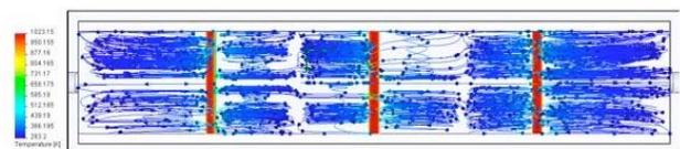
Fig. 9. Computational Fluid dynamics (CFD) analysis of the convection flows inside of the reactor. The reactor cavity dimensions are 40 mm x 50 mm x 300 mm. The long lateral walls are adiabatic. (Reactor top view)
