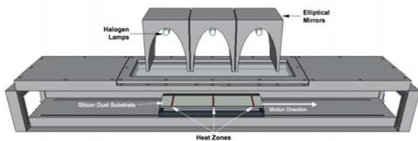
Fig. 2. Cut view of the CVD system schematic
