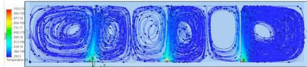
Fig. 4. Computational Fluid dynamics (CFD) analysis of the convection flows inside of the reactor. The reactor cavity dimensions are 60 mm x 60 mm x 300 mm. The ratio between the distance from the sample to the quartz window and the distance between heat regions (80 mm) is 3/4. The fluid injection is made from the orifice on the left wall. (Reactor side view)
