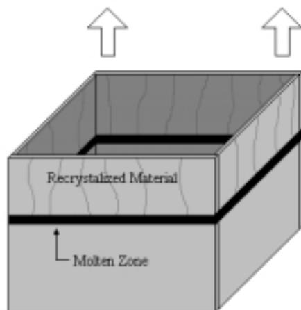
**Figure 1:** Schematic diagram of the Closed Molten Zone technique, where silicon is recrystallised into a square tube.
