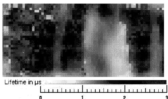
**Figure 4:** Carrier lifetime map of a closed molten zone sample (R5B) as measured by Microwave Reflectance Decay. Area displayed is about 220mm<sup>2</sup> and the average lifetime is about 1.7  $\mu\text{s}$ , consistent with the average diffusion length of 83  $\mu\text{m}$  obtained in similar conditions (no bias light).
