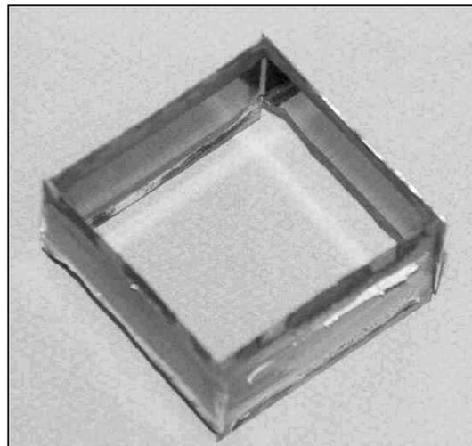
**Figure 2:** Top view of a 50 mm wide recrystallised silicon tube.
