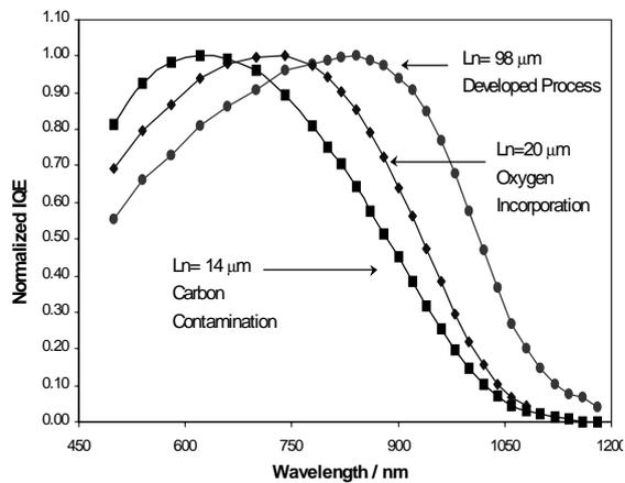
**Figure 3:** Normalised internal quantum efficiency of simple test cells made from silicon sheet obtained in different growth conditions. The degradation due to carbon contamination and oxygen incorporation is compared with the result for the developed CMZ process.
