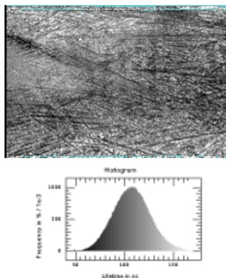
**Figure 5:**  $\mu$ -PCD measurement of an as grown RGS wafer (11x8 cm<sup>2</sup>, no surface passivation).
