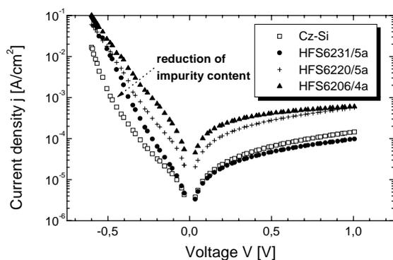
**Figure 4:** Dark current-voltage characteristics of solar cells based on RGS ribbons in comparison to a mono Cz Si solar cell. Impurity level: 06206/4aL: medium; 06220/5aL: low; 06231/5aL: very low. The reduction of the impurity content of the RGS ribbons leads to a decrease of the dark current density of the corresponding solar cell.
