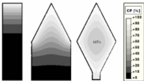
**Figure 1:** Collection probability CP for minority charge carriers generated in the base of solar cells with different surface texture (maximum cell thickness  $300\ \mu\text{m}$ , diffusion length  $L_{\text{diff}} = 50\ \mu\text{m}$ ).
