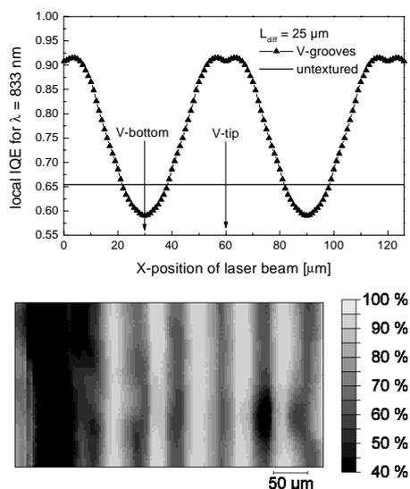
**Figure 6:** Top: Simulated local IQE at 833 nm for a flat and mechanically V-textured solar cell with  $L_{diff} = 25 \mu m$ . Light entering in the V-tips results in an increased IQE. Bottom: Measured local IQE at 833 nm of a textured RGS solar cell with  $L_{diff}$  about 25 μm. An excellent agreement between simulation and measurement is visible.
