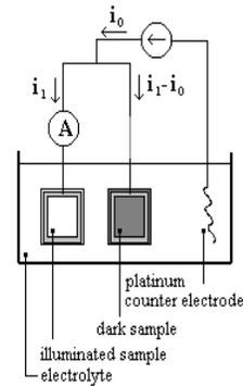
Fig. 2: Modified experimental set-up to allow separate measurement of currents in dark and illuminated areas.
