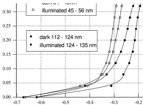
Fig. 1: I-V curves obtained for  $n^+$  phosphorus diffused silicon in successive dark and illuminated sweeps, at etched depths as indicated.
