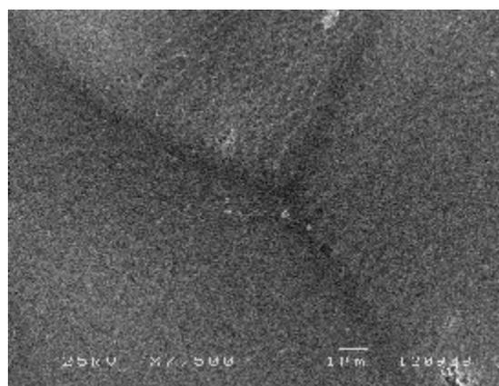
Fig.2 – SEM pictures showing the structure of the ribbon before and after ZMR. Top photograph: as grown CVD pre-ribbon; Bottom photograph: after ZMR.
