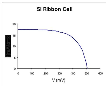
Fig. 3- I-V curve of our best test cell.
