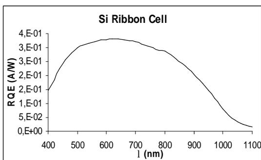
Fig.4- Spectral response of one of these test cells.
