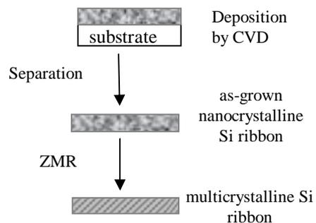
Fig.1- Process sequence of the SDS technique.
